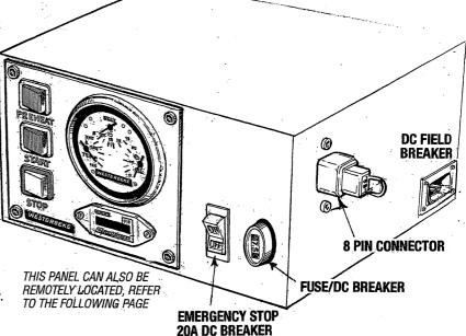
**Engine Oil Pressure:** Oil Pressure (psi) may fluctuate depending on the generator load but should range between 35 to 55 psi.
