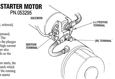
To test the ignition circuit, locate the ignition(s) terminal (it is one of the small terminal studs and is wired to the ignition circuit). Use a screwdriver, don't touch the blade, to jump from that ignition terminal to the positive battery connection terminal on the solenoid.
