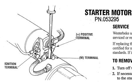
Test again by jumping the two large terminal studs. Hold the screwdriver blade firmly between the studs. Do not allow the screwdriver blade to touch the solenoid or starter casing, this would cause a short.
