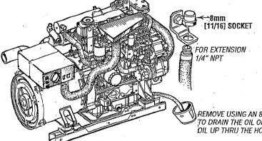
3. Filling the Oil Sump. Add new oil through the oil filler cap on the top of the engine or through the side oil fill. After refilling, run the generator for a few moments while checking the oil pressure. Make sure there is no leakage around the new oil filter or from the oil drain system, and stop the engine. Then check the quantity of oil with the lube oil dipstick. Fill to, but not over the high mark on the dipstick, should the engine require additional oil.
