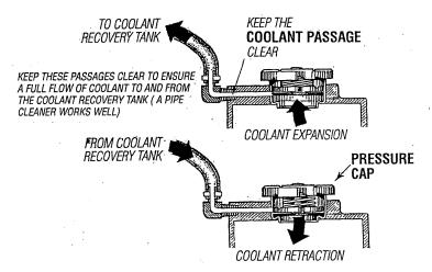
**NOTE:** Periodically check the condition of the manifold pressure cap. Ensure the upper and lower rubber seals are in
